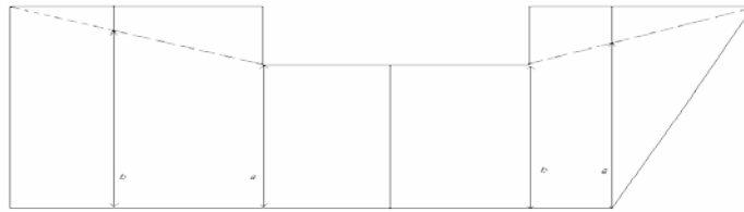
Figure III/21-3 Freeboard Measurement Boat with Stepped Bulkhead Deck and a Porthole below the Bulkhead Deck
