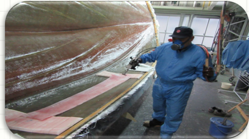
Using a Chopper Gun with Resin to the RFM
