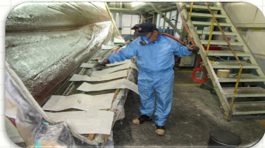
Using a Chopper Gun with Resin to the RFM
