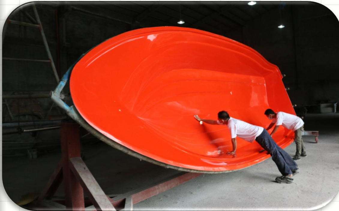
APPLYING RELEASE WAX TO THE MOULD
