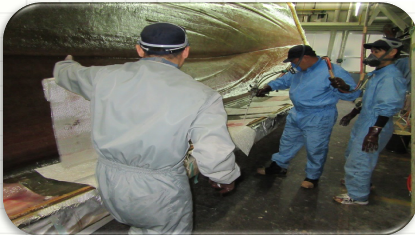
Using a Chopper Gun with Resin to the RFM
